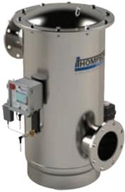
A water strainer ensures you have the highest quality water for use with your Sioux chiller. Strainers include an Automatic Timer Flush Package with PLC and pressure transducers to monitor the differential pressure. Stainless steel construction with either a bolted or clamp lid (depending on model) for access to the screen, multiple sizes for different max flow rates, and NEMA 4X electrical enclosure. Requires 115V/1Ph/60Hz electrical connection for operation.
