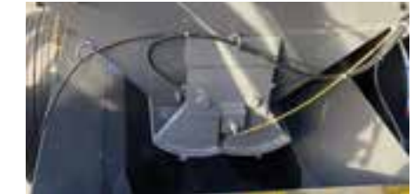
PROXIMITY SWITCHES ON HEAVY-DUTY GATES
