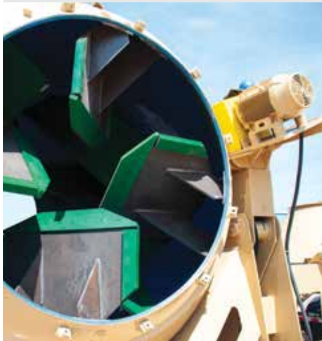
WRAP-AROUND POLY-LINED AR-400 STEEL BLADES & TWIN 75 HP MOTORS
