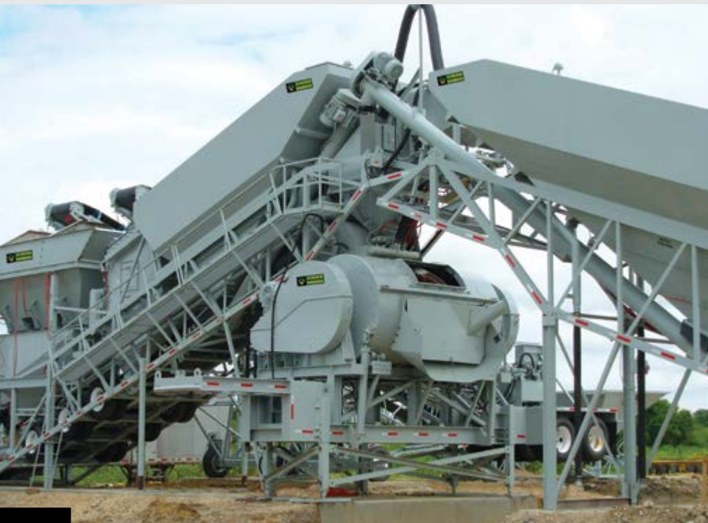
HT PAIRED WITH HORIZONTAL SHAFT MIXER
