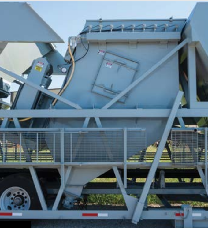
IN-TRUSS DUST COLLECTOR
