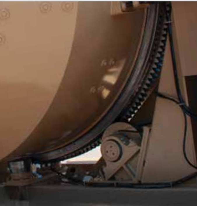
HEAVY-DUTY DRUM ROLLERS & FORGED RING GEAR
