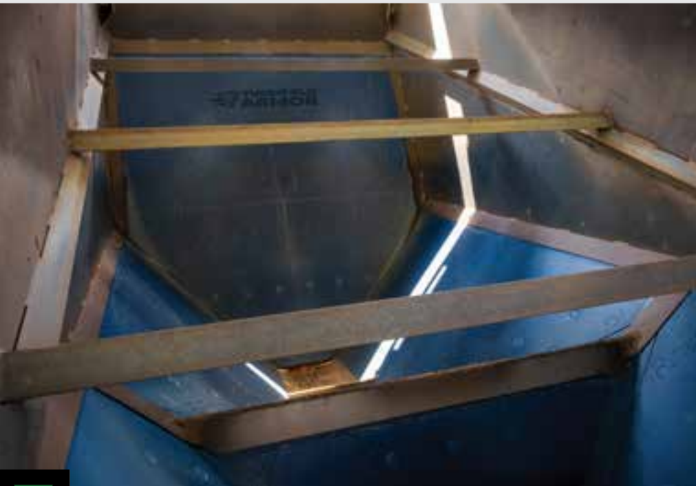
FULL COVERAGE OF THE TURBO-FLO ARMOR™ LINERS
