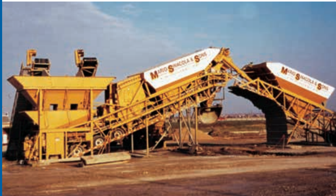
HT-SERIES BATCH PLANT AND HCA AUXILIARY SILO
